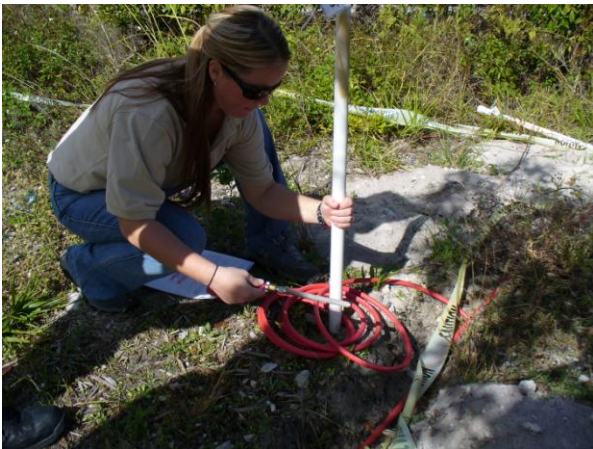
Photo of the proprietary sparger being inserted into the injection well.
