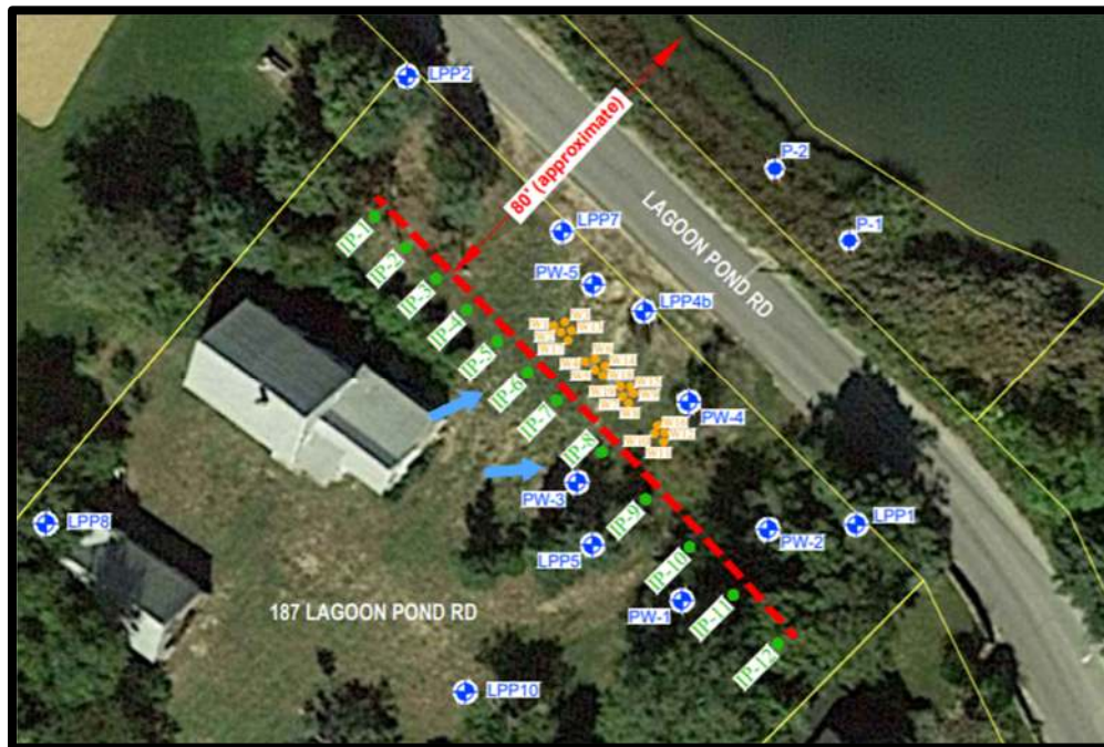
Figure 33. Lagoon Pond Road Site As Built Map Showing Final Placement of the PRB and Multi-Level Monitoring Wells (SMAST 2023)
